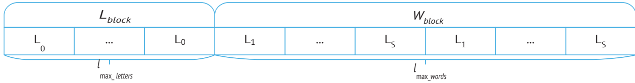
Figure 3. Structure of synchronisation block and data block
